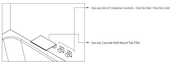
2) Wall Mount Tub Filler w/Thermostatic Temperature Control + Volume control
