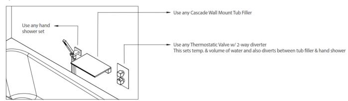
2) Wall Mount Tub Filler With Hand Shower - simultaneous flow between hand-shower and tub filler
