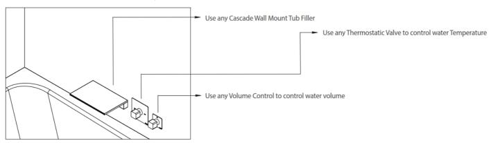
3) Wall Mount Tub Filler w/Thermostatic Valve w/Integrated Volume Control
